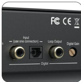
Digital Inputs & Loop Output
